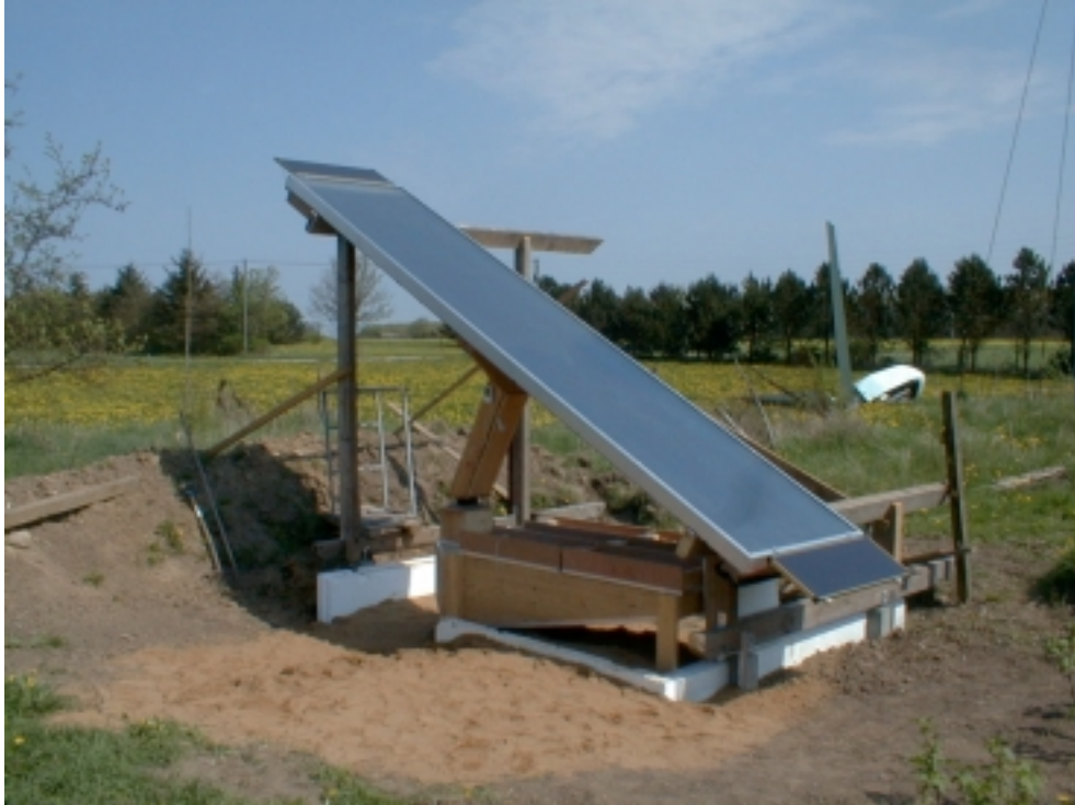
Figure 4.2. Photo of the first design of the solar crop dryer – one unit.
