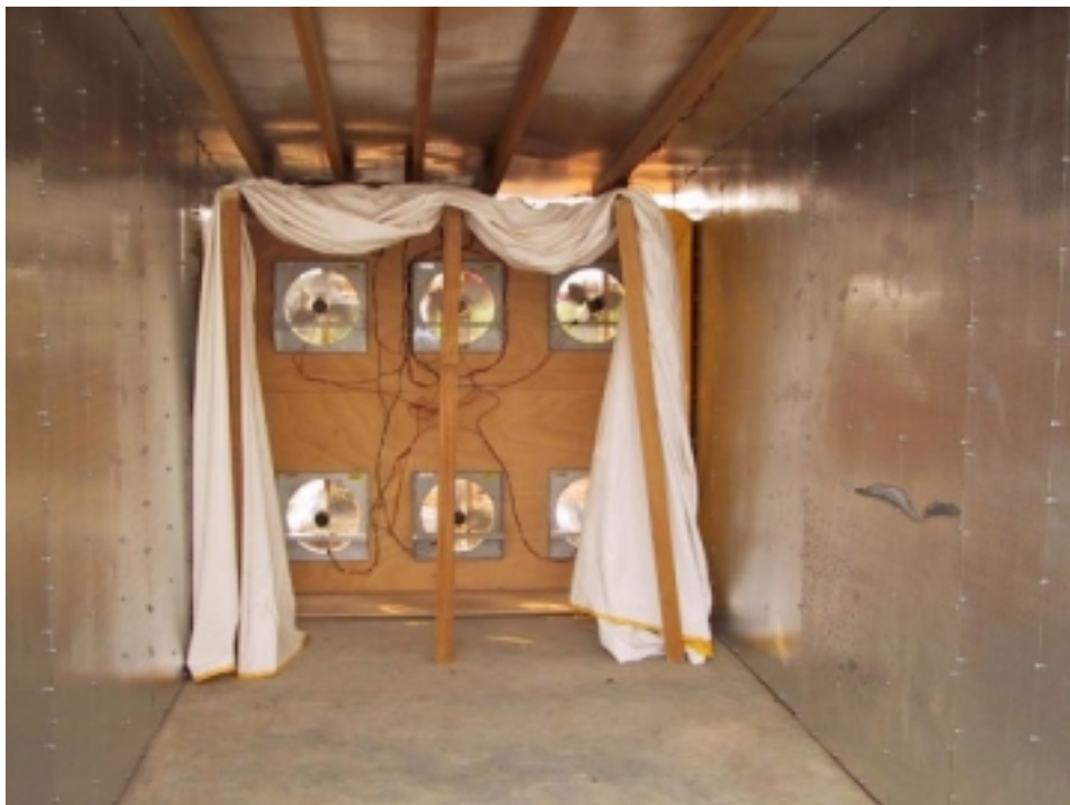
Figure 5.2. The pressure chamber of the forced open air dryer with fans and the tarpaulin.
